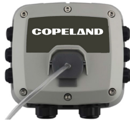
Figure 5-1 - Calibration Adapter Fitting
